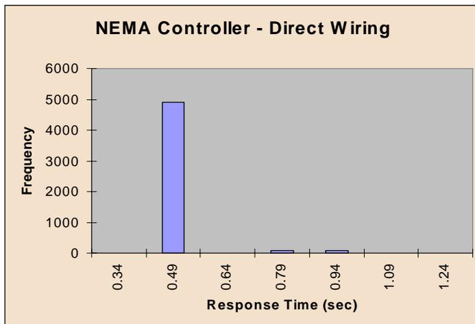
The base line response time measurements for the TRAP and the NEMA protocols summarized in the two histogram graphs. The above graphs clearly indicate the response times for the traffic controllers are deterministically contained within 1 second. However, the bulk of the responses are much less than ½ second.
