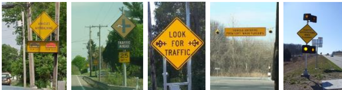
Figure 1 Intersection Conflict Warning Systems
