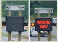
Vehicle-activated "Blank Out" DMS (Source: Cooner et al., 2004)
