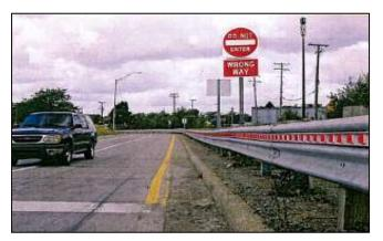
Red Delineators on Guardrail along Exit Ramp (Source: Morena and Leix, 2012)
