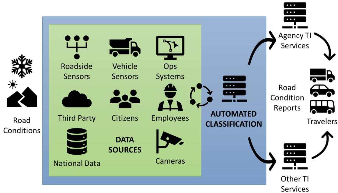
**Figure 1: Operational Concept for Automated Classification of Road Conditions**
