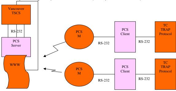
Each TC receives a unique IP address from the service provider and these IP addresses are mapped to the controllers configuration in the system database.
