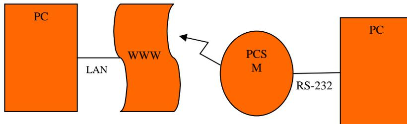
Open source IP protocol testing tools were used to establish the characteristics of the 1xRTT PCS communications. These tests were conducted using standard PC hardware and software independent of any traffic signal control applications. These tests measured throughput of the 1xRTT network utilizing UDP and TCP/IP which were measured at 40 and 30 kb/s, respectively. Appendix A provides additional test result data.
