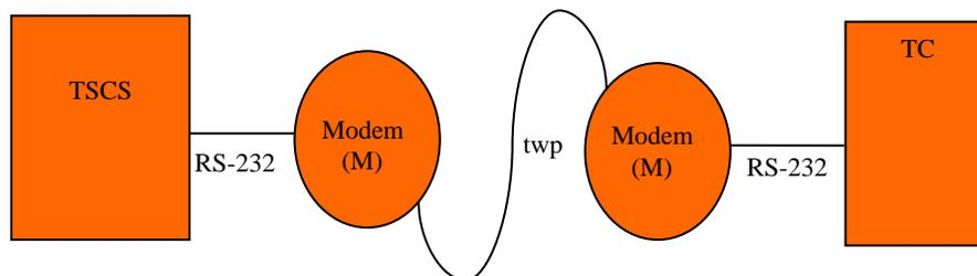
Normal application level poll packets transmitted from the TSCS are received by the TC, processed and a response to the poll request is returned. The baseline response times were measured at the TSCS. These times, represent the total time from transmission of the poll request to the reception of the response.
