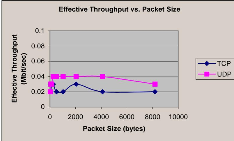
The above graph is a sample measurement of the raw sustained throughput for the 1xRTT communications services. This establishes a base line measurement for the communications over the 1xRTT. For UDP traffic, 40 Kbps sustained data rates were observed. For TCP/IP, greater than 30 Kbps sustained data rates were observed.
