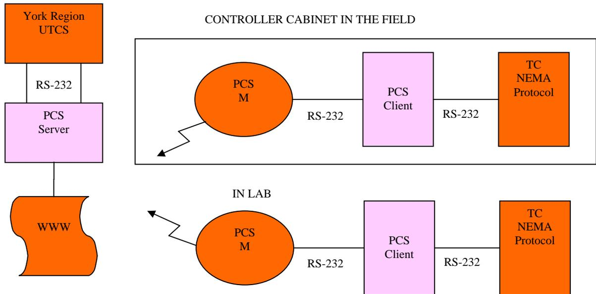
The testing included utilizing the traffic monitoring functionality of the central system such as status polling and uploading of the current configuration information in the TC. Control operations were only exercised with the presence of support personnel at the TC field cabinet site for safety reasons. Data was collected over several days from the live TC in the field.
