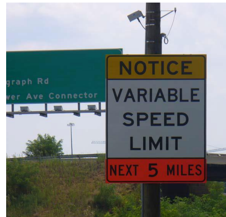
VSL Alerting Drivers to the Beginning of VSL Zone in Virginia
