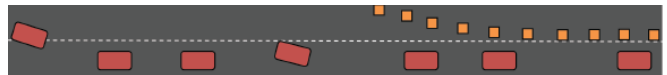
Early Merge Concept Diagram (Source: ATSSA Guidance for the Use of Dynamic Lane Merging Strategies)
