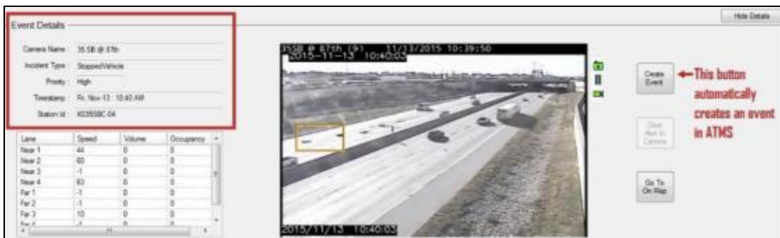
Figure 5: Kansas City Scout Alert TrafficVision API Integration with ATMS Software Easy Button (Courtesy of Kansas City Scout)
