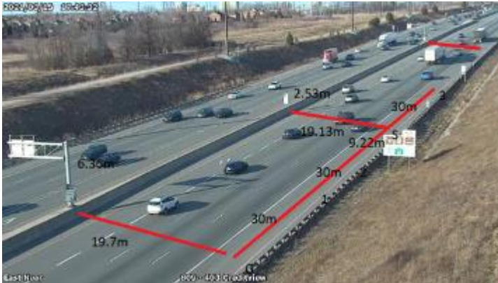
Figure 6: Lane marking measurements for Bosch AID (Photo courtesy of MTO)
