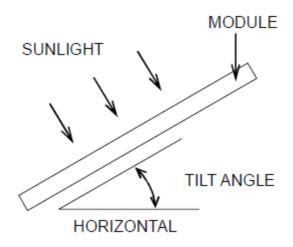
Figure 25: Solar panel tilt angle (source ref. [5]).
