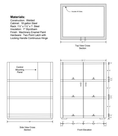
Figure 17: Battery cabinet specification.
