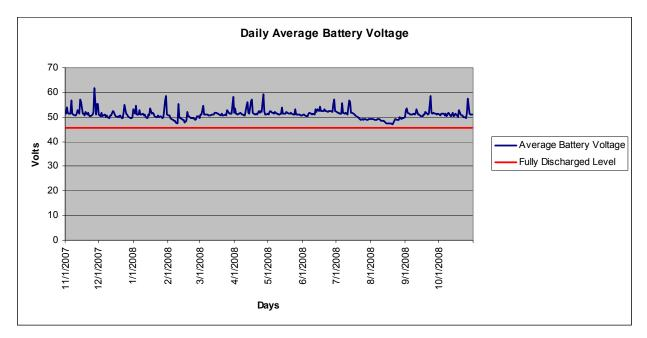
Figure 30: Daily average battery voltage from Nov. 2007 - Oct. 2008.
