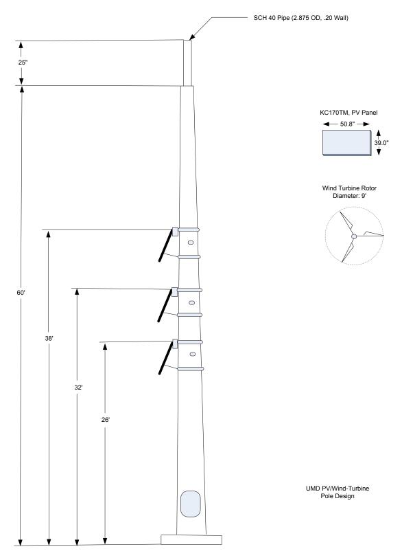
Figure 9: Mounting pole design specification.
