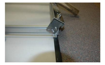
5. Prepare the second U-channel by attaching the two shorter legs. The legs should be mounted outside the L-brackets as shown.
