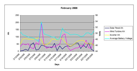
Figure 33: Ah totals for solar, wind, inverter, and average battery voltage for February 2008.
