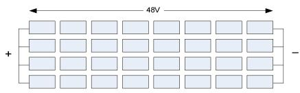
Figure 7: Battery connections for the battery bank.
