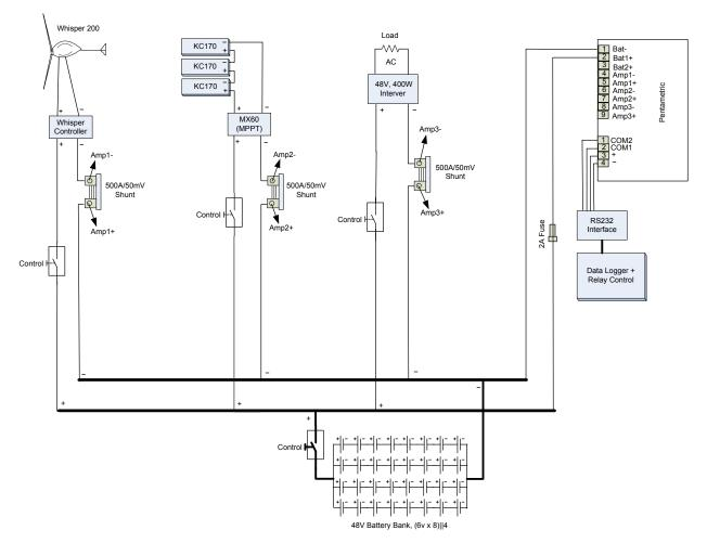
Figure 16: Solar/Wind HRPG circuit design.
