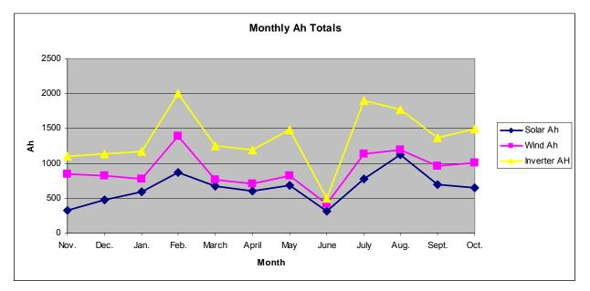
Figure 28: Monthly Ah totals for solar, wind, and inverter from Nov. 2007 – Oct. 2008.
