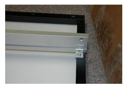
3. Mount L brackets to both U-channels using 9/16" bolts and nuts. At this point, loosely tighten the bolts and nuts.
