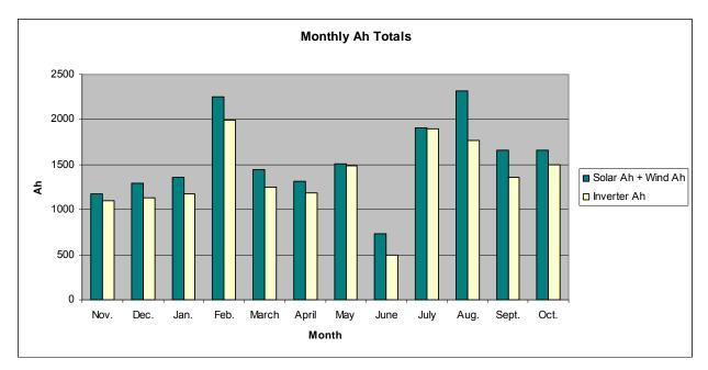
Figure 29: Monthly Ah totals for solar + wind and inverter from Nov. 2007 – Oct. 2008.
