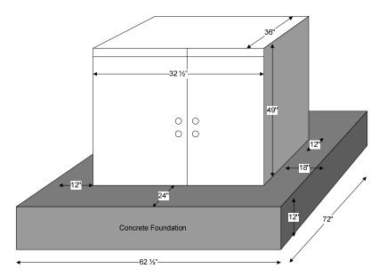
Figure 18: Battery cabinet and foundation dimensions.
