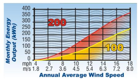
Figure 8: Monthly energy output of Air-X per annual average wind speed (source ref. [6]).
