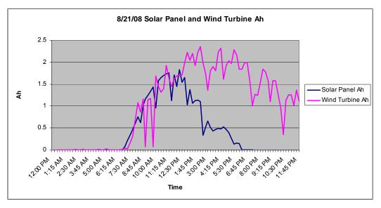
Figure 32: Hourly solar and wind Ah on 8/21/08.
