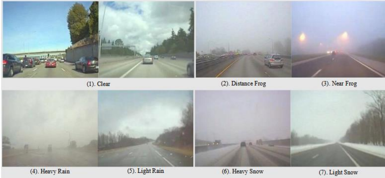
Figure 6. Seven categories of weather used to train AI in Wyoming. Source: Wyoming DOT . 16
