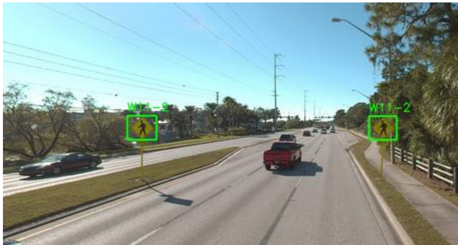
Figure 7. AI can Identify Road Signing in Support of Asset Management Practices. Source: iEngineering . 18
