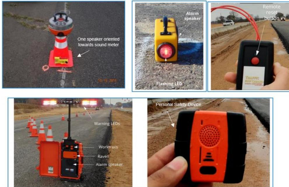
**Figure 3-4 Examples of Different Work Zone Intrusion Alarm Technologies (Source: FHWA)**
