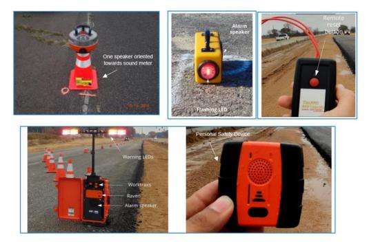
Figure 3-4 Examples of Different Work Zone Intrusion Alarm Technologies (Source: FHWA)
