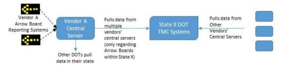
Another option is that DOTs would operate a proxy server to enable Arrow Boards to report directly to the proxy server, or to communicate via. Vendor operated central servers. This would allow the TMC Systems to pull data from their own Proxy Server.
