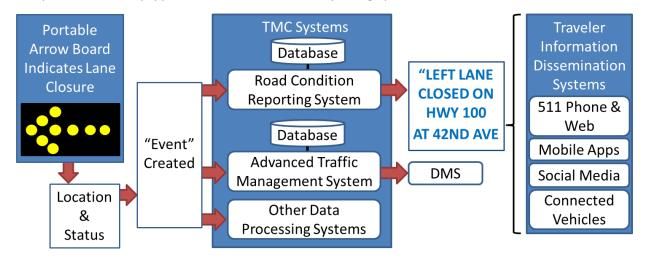
Figure 1: The systems of interest for these System Requirements include Portable Arrow Boards and TMC Systems, which encompass Road Condition Reporting Systems, Advanced Traffic Management Systems, and traveler information dissemination systems.
