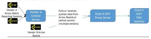
Figure A-2: Illustration of Possible Options for Arrow Board Reporting Systems
