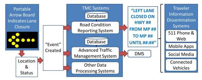
Figure A-1: The systems of interest for this ConOps include Portable Arrow Boards, Road Condition Reporting Systems, Advanced Traffic Management Systems, and traveler information dissemination systems.
