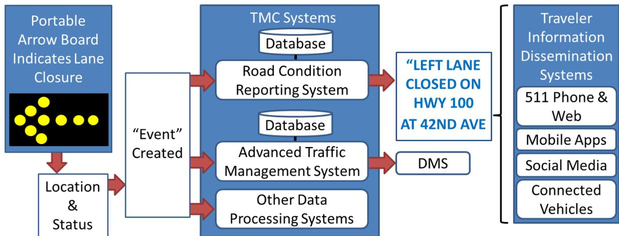
**Figure 1: The systems of interest for these System Requirements include Portable Arrow Boards and TMC Systems, which encompass Road Condition Reporting Systems, Advanced Traffic Management Systems, and traveler information dissemination systems.**
