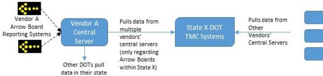
Another option is that DOTs would operate a proxy server to enable Arrow Boards to report directly to the proxy server, or to communicate via Vendor operated central servers. This would allow the TMC Systems to pull data from their own Proxy Server.
