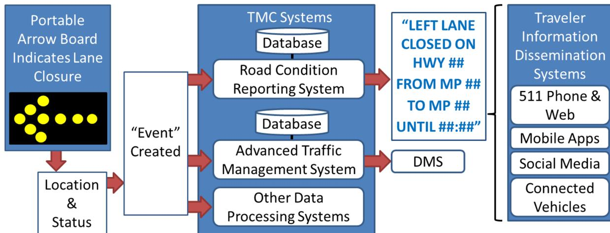
**Figure A-1: The systems of interest for this ConOps include Portable Arrow Boards, Road Condition Reporting Systems, Advanced Traffic Management Systems, and traveler information dissemination systems.**
