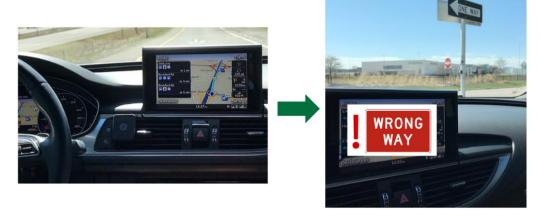
Figure 1: Concept - Wrong-Way Alert from In-Vehicle Navigation
