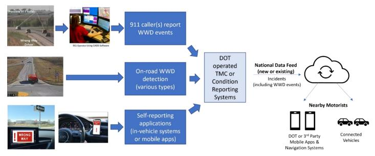
Figure 1: Wrong-way Driving (WWD) Events Communicated Through a National Incident Data Feed
