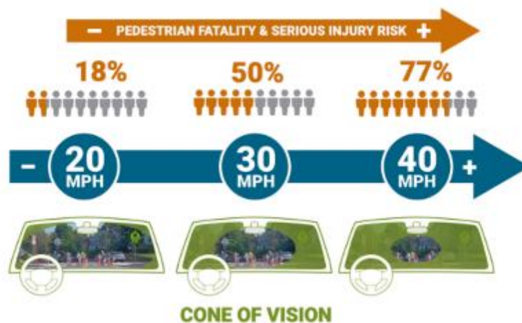
Figure 8: Average Risk of Pedestrian Fatalities and Injuries at Increasing Speeds and Cone of Vision (Source: Porter et al. 5 )
