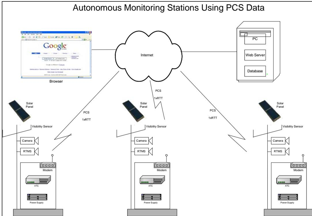
Figure 2-1 System Design Diagram
