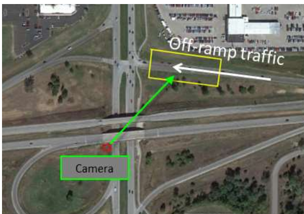
Figure 2-10: Deployment Site #2 (90 degree detection)
