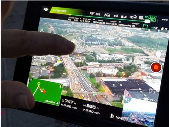
Figure 4.7 Screenshot of Live Stream Videos from Drones to Assess Traffic Congestion During Construction (Source: [Innovation Spotlight: NJDOT UAS Program](#))
