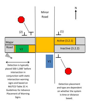
Illustration is not drawn to scale and is shown from the minor road, northbound vehicle (V1) perspective. Warning signs may be placed on the far-side corner (1) from STOP or far-side opposite corner (2) from STOP as a supplement to (1). Signing has also been suspended above the minor road in the intersection but the placement has since been found less effective through a safety effectiveness evaluation conducted by the North Carolina Department of Transportation.
