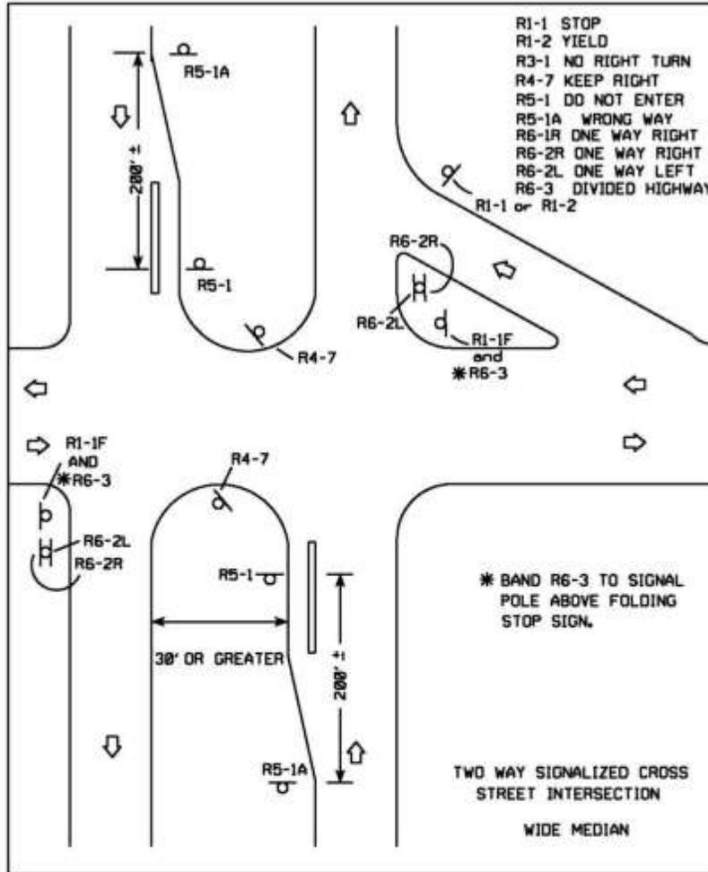
FIG. 16 WRONG WAY SIGNING RELATIVE TO DIVIDED HIGHWAY.
