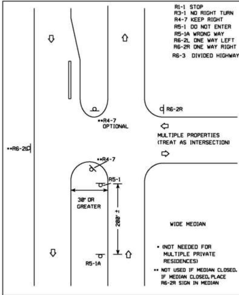
FIG. 11 WRONG WAY SIGNING RELATIVE TO DIVIDED HIGHWAY.
