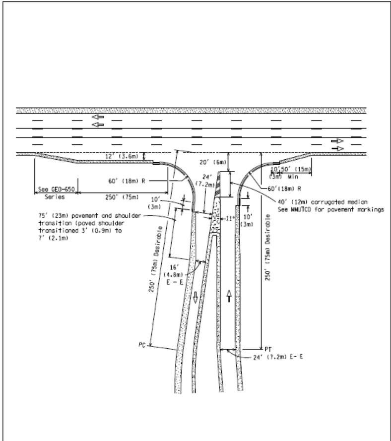
At unsignalized ramp terminals, it is desirable to redirect the left turns right from the ramp to an adjacent directional crossover when the median width can accommodate truck traffic (WB-65).
