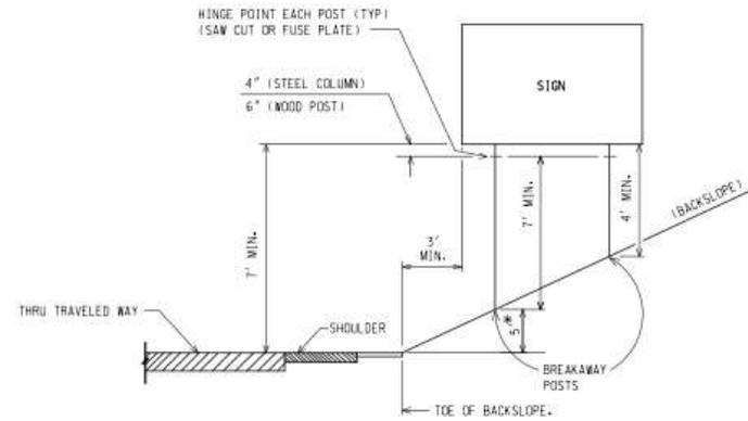
\* IN DEPRESSED SECTIONS WITH 3:1 OR STEEPER BACKSLOPE, IF THE FRONT (TRAFFIC SIDE) POST CANNOT BE LOCATED AT 7' ABOVE SHOULDER ELEVATION, THEN A 3' MINIMUM OFFSET FROM THE TOE OF SLOPE SHALL BE MAINTAINED AND THE SIGN PROTECTED WITH AN APPROVED BARRIER. SEE GENERAL NOTE 5.
