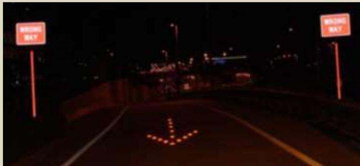
**Red Reflective Tape on Sign Posts, Signs on Both Sides of Ramp**
