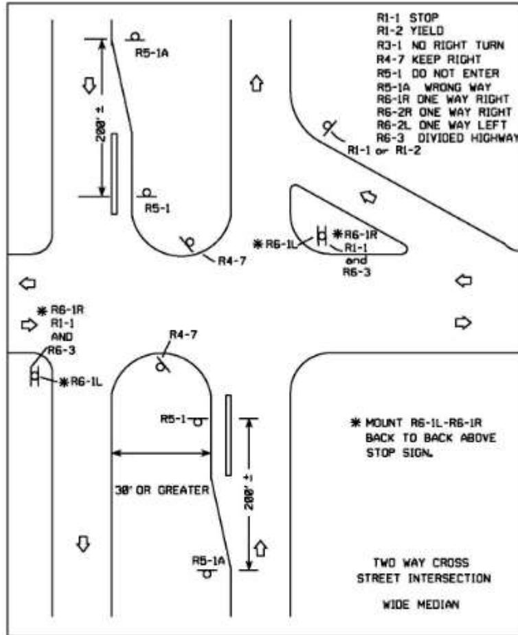
FIG. 1 WRONG WAY SIGNING RELATIVE TO DIVIDED HIGHWAY.
