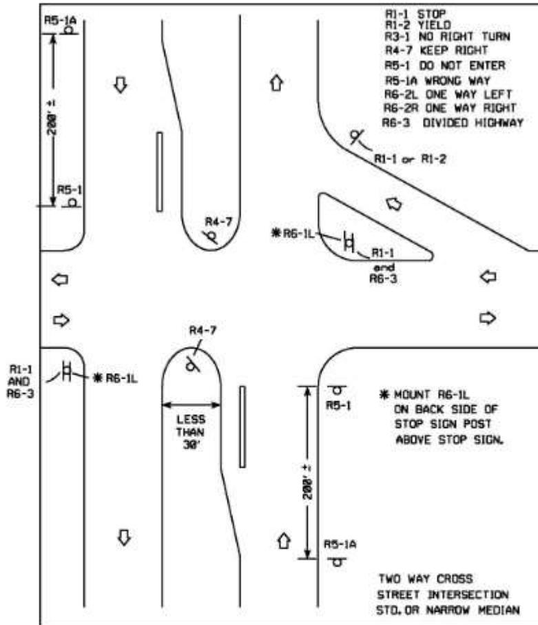
FIG. 2 WRONG WAY SIGNING RELATIVE TO DIVIDED HIGHWAY.
