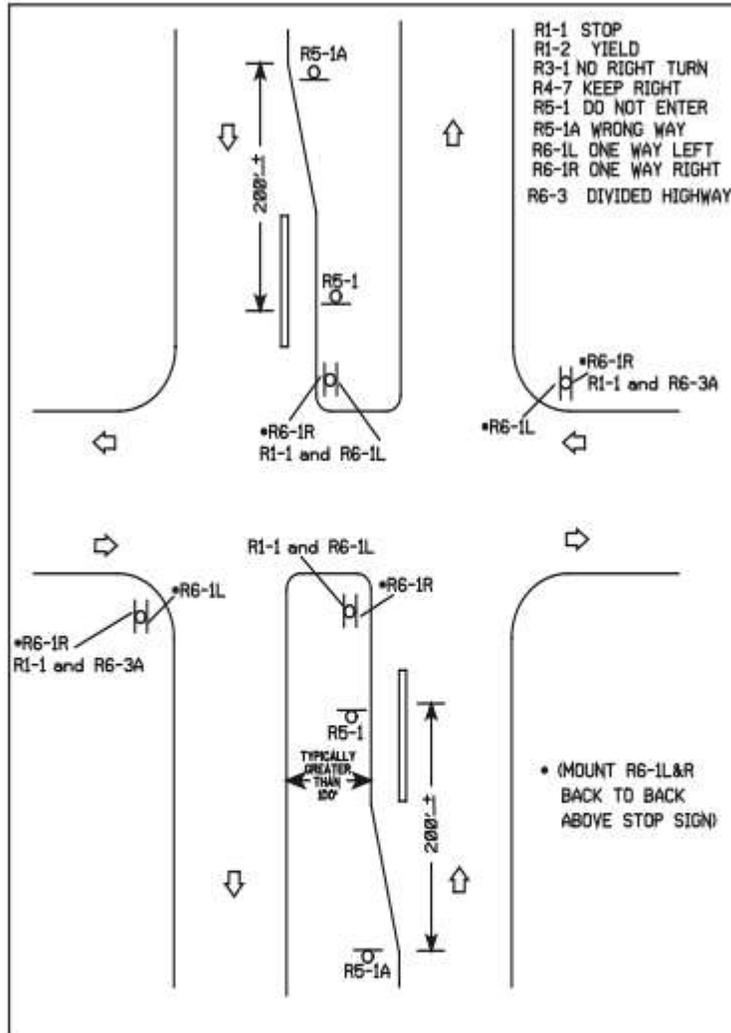
FIG. 15 WRONG WAY SIGNING RELATIVE TO DIVIDED HIGHWAY.
