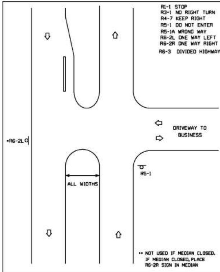
FIG. 10 WRONG WAY SIGNING RELATIVE TO DIVIDED HIGHWAY.
