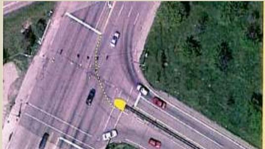
**Skip Lines to Guide Drivers onto Entrance Ramp, Stop Bar at End of Exit Ramp**
