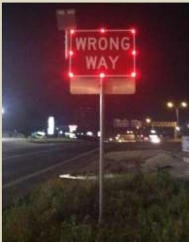
**LEDs at WRONG WAY Sign Border, Flash Continuously at Night & Low Light**
