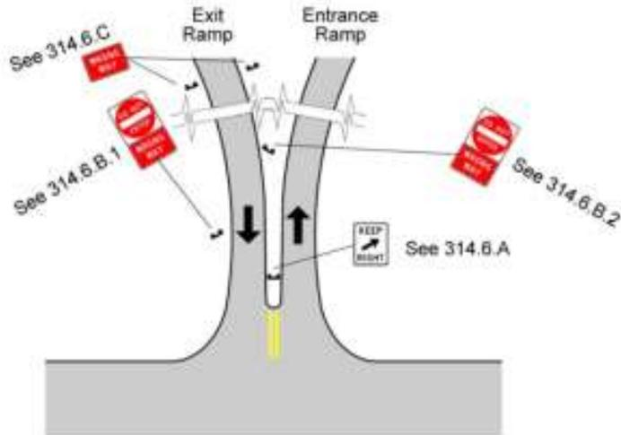
**Figure 314-H. Wrong Way Signing at Partial Cloverleaf Traffic Interchange**
