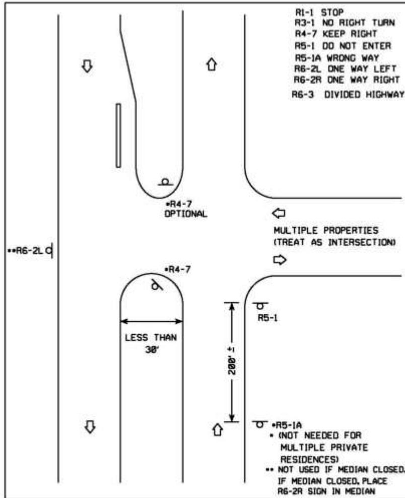
FIG. 12 WRONG WAY SIGNING RELATIVE TO DIVIDED HIGHWAY.
