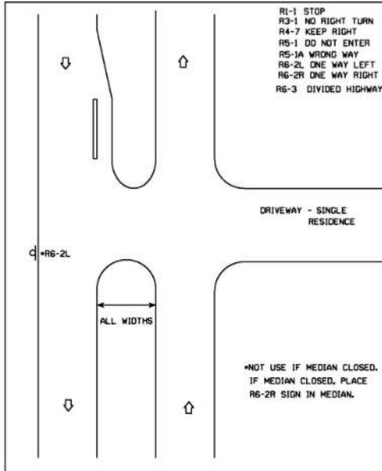
FIG. 9 WRONG WAY SIGNING RELATIVE TO DIVIDED HIGHWAY.
