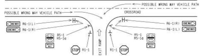
TYPICAL LOCATION OF R5-1 & R5-1c ON EXIT RAMPS. THESE SIGNS SHOULD BE TURNED APPROXIMATELY 20 DEGREES FROM THE CROSSROAD TO FACE THE PATHS OF POSSIBLE WRONG WAY VEHICLE MOVEMENTS.
