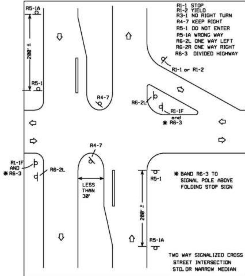
FIG. 17 WRONG WAY SIGNING RELATIVE TO DIVIDED HIGHWAY.
