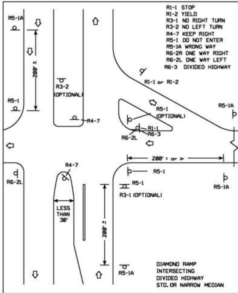
FIG. 4 WRONG WAY SIGNING RELATIVE TO RAMP.
