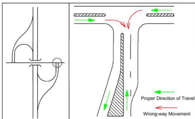
**Figure 2: Potential Wrong-way Movements in Partial Cloverleaf Interchanges**
