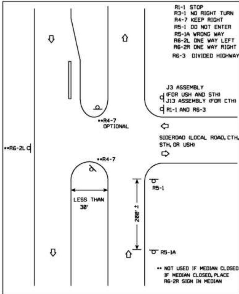
FIG. 7 WRONG WAY SIGNING RELATIVE TO DIVIDED HIGHWAY.
