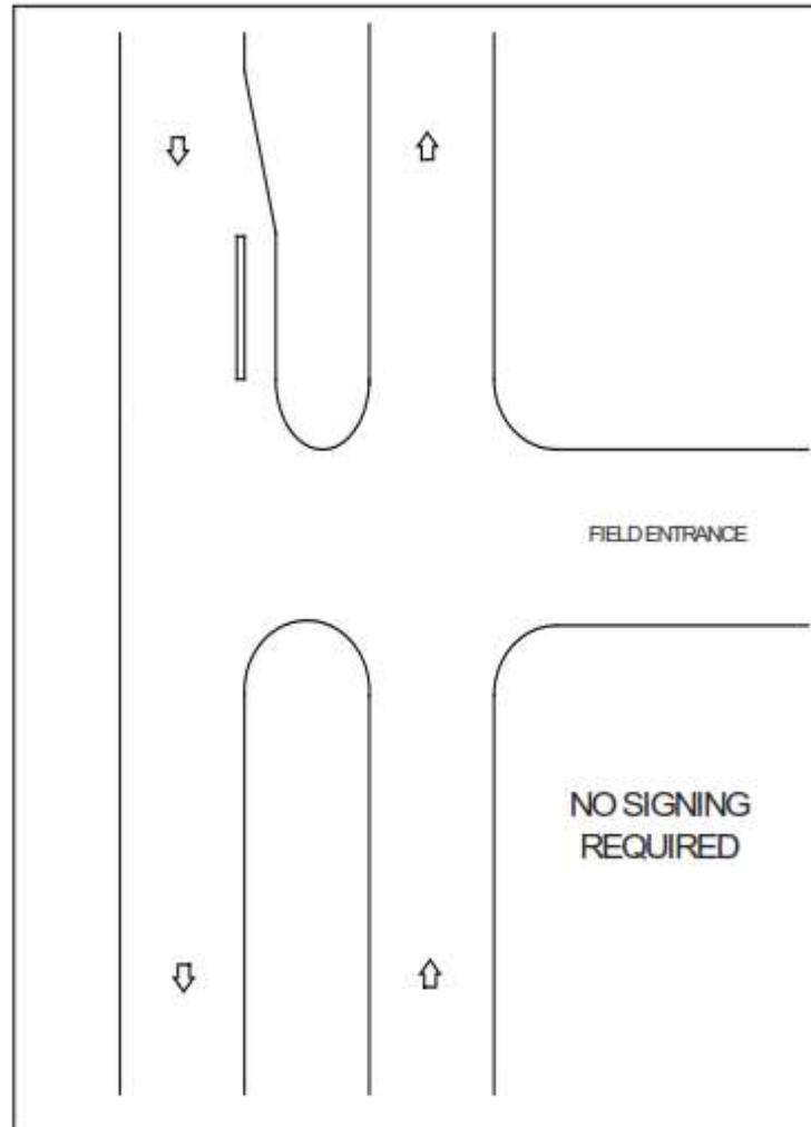
FIG. 13 WRONG WAY SIGNING RELATIVE TO DIVIDED HIGHWAY.
