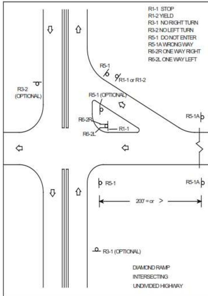
FIG. 5 WRONG WAY SIGNING RELATIVE TO RAMP.
