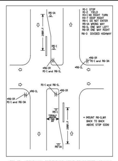
FIG. 15 WRONG WAY SIGNING RELATIVE TO DIVIDED HIGHWAY.
