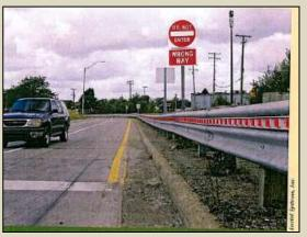
Red Delineators on Guardrail along Exit Ramp (Source: Morena & Leix, 2012)
