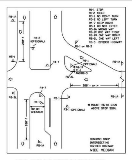
FIG. 3 WRONG WAY SIGNING RELATIVE TO RAMP.
