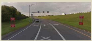
Signs on Both Sides of Ramp; Two Signs on the Same Post (Source: Provided by Ohio DOT)
