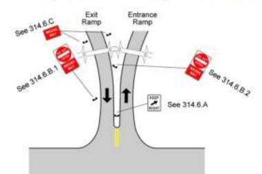
Figure 314-H. Wrong Way Signing at Partial Cloverleaf Traffic Interchange (with right turn island)
