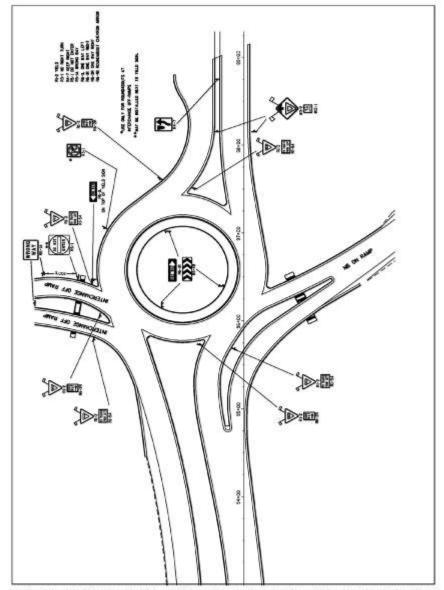
FIG. 14 WRONG WAY SIGNING RELATIVE TO ROUNDABOUT
