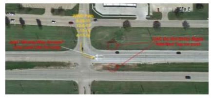
Improvements at Linn Street and U.S. 30 Intersection: DNE Signs on Both Sides of Highway, Wrong-Way Arrow Pavement Markings (Source: Iowa DOT)
