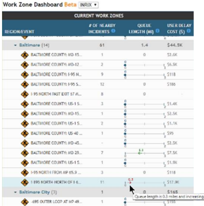
Figure 4. Work Zone Performance Monitoring Dashboard developed by the University of Maryland-Center for Advanced Transportation Technology Laboratory (UMD-CATT Lab) for the Maryland State Highway Administration (SHA).
