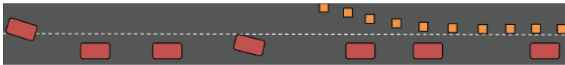
Figure 2: Early Merge Concept Diagram (source: ATSSA Guidance for the Use of Dynamic Lane Merging Strategies 1 )
