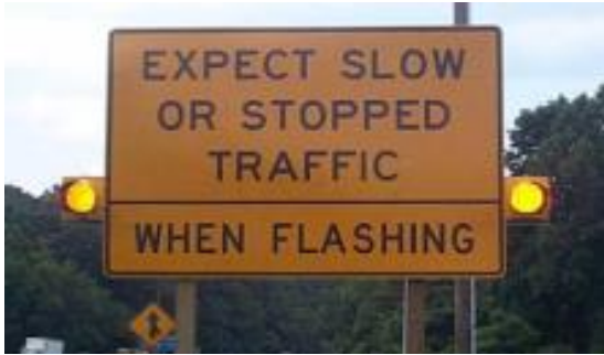
Figure 9: Static Queue Warning Sign with Flashing Beacons in Asheville, North Carolina
