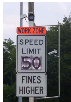
Figure 13: VSL Sign Posted in a Work Zone in Virginia
