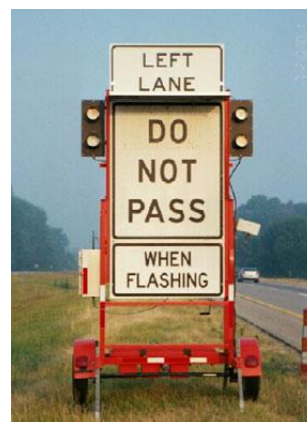
Figure 6: Dynamic Sign and Trailer Used in Michigan 20
