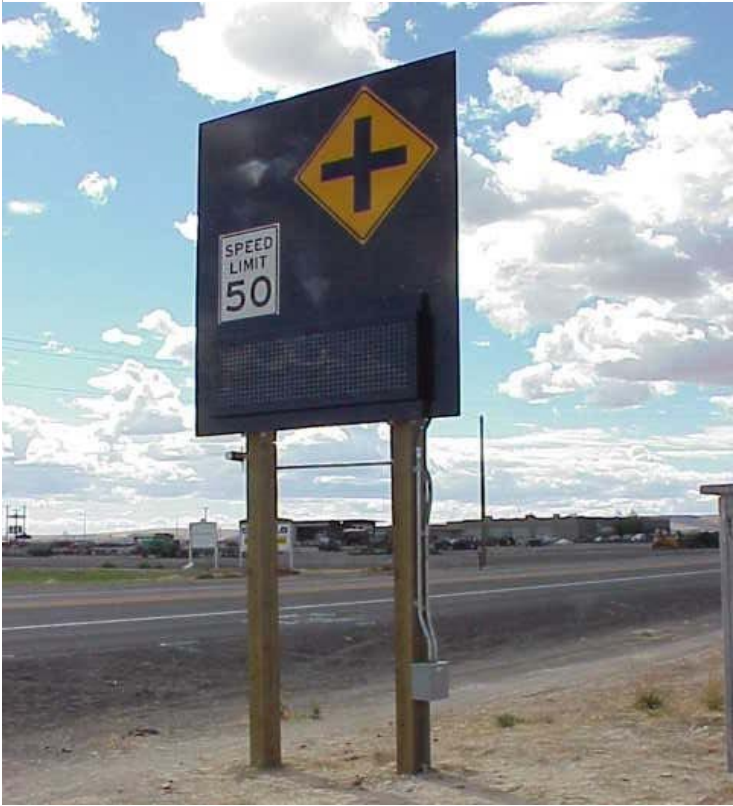
Figure 15 Combination Speed/Warning Sign – Othello, WA
