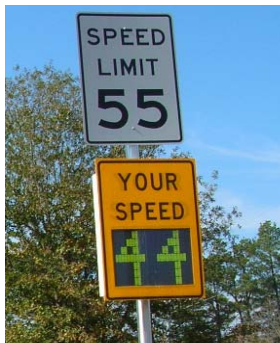
Figure 14 Dynamic Speed Sign
