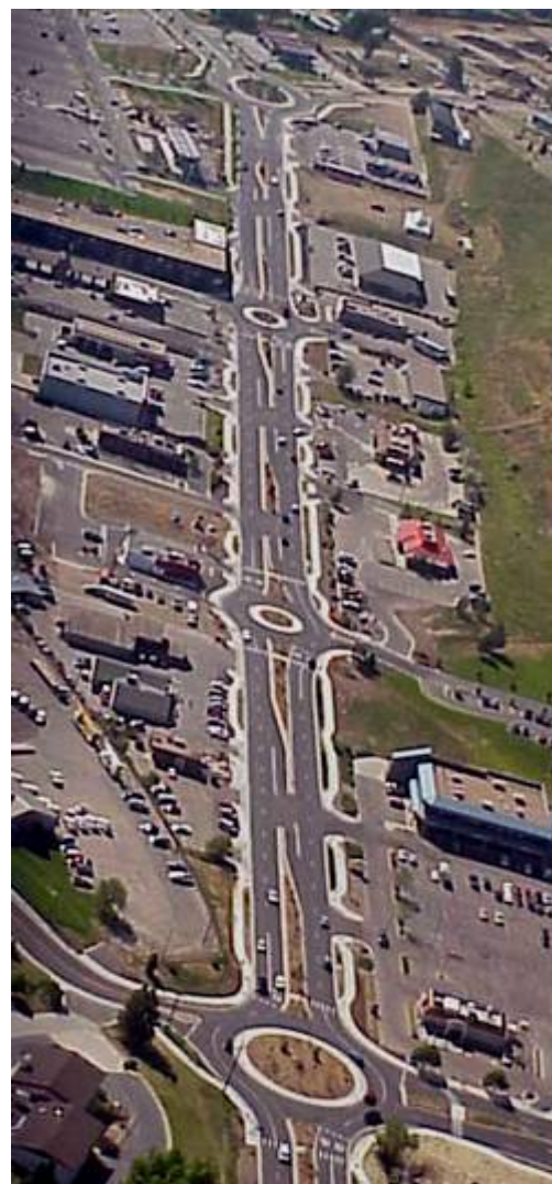
Figure 35 Arterial Multi-Lane Roundabouts Used For Access Management (Golden, Colorado)
