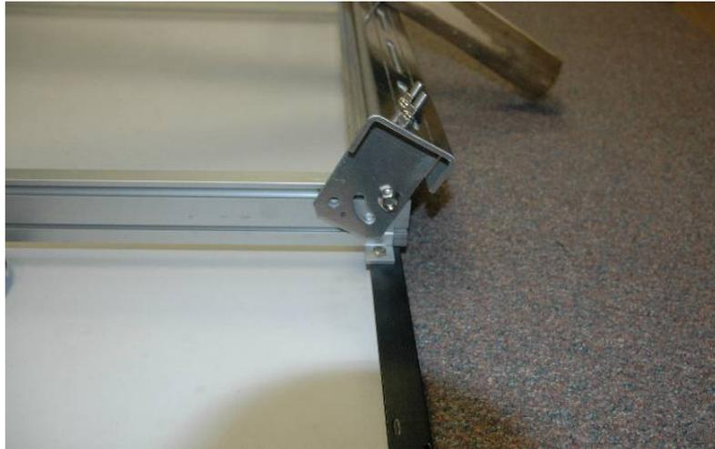
5. Prepare the second U-channel by attaching the two shorter legs. The legs should be mounted outside the L-brackets as shown.
