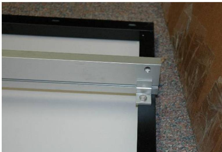
3. Mount L brackets to both U-channels using 9/16" bolts and nuts. At this point, loosely tighten the bolts and nuts.
