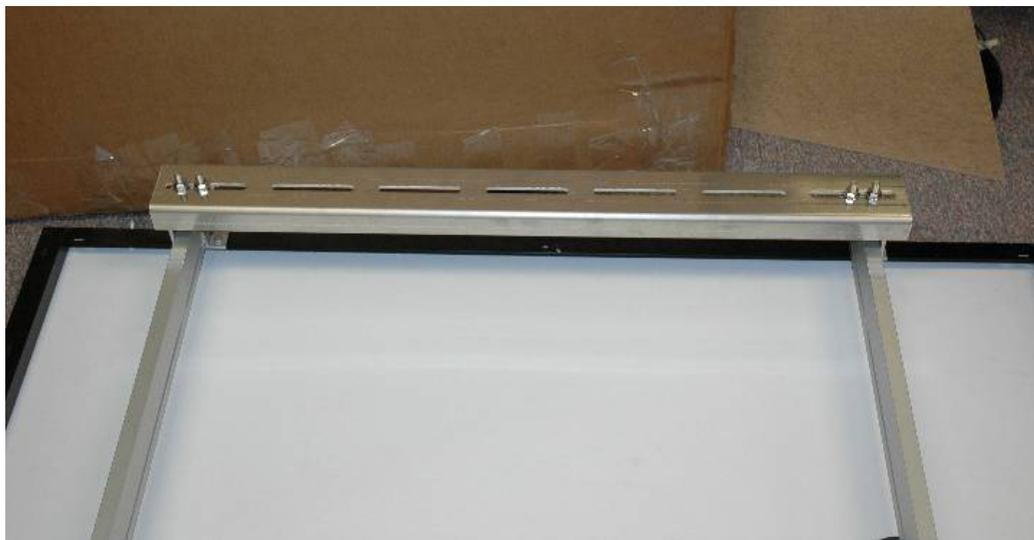
Use the small, outside hole on the L-bracket on both ends as shown in the picture below.
